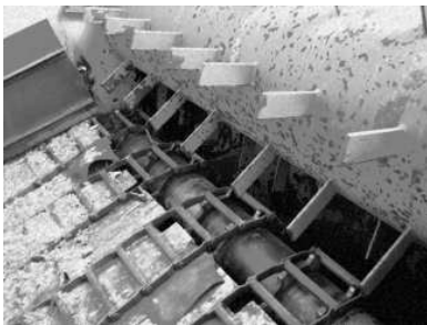
Discharge End with Spike Roll
